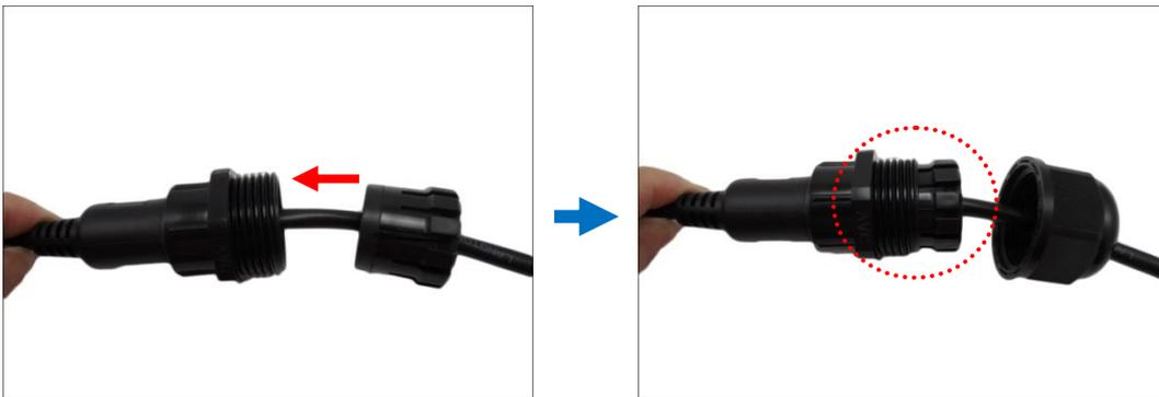
9. Attach the clamping nut to the cable gland body. Make sure the clamping nut is tightly secured and the rubber is squeezed in to avoid water leakage.
