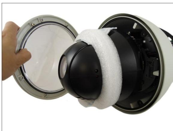
**NOTE:** The cover is attached to the camera by a metallic wire strap; do not abruptly lift the cover.
