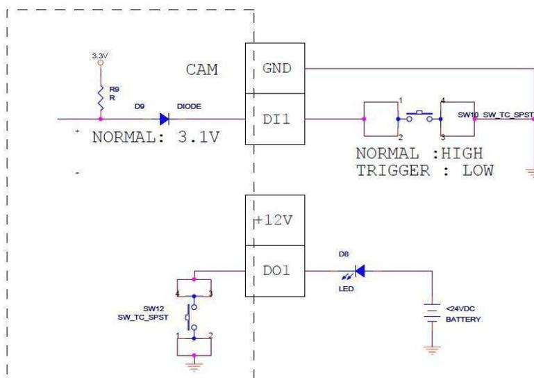
Consequently, to connect a second DI or DO device, use the Black (GND) and Green (DI2) cables to connect the second DI device, and the Red (12V) and Blue (DO2) cables for the second DO device.
