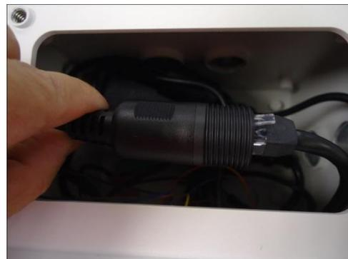
3. Secure the flex conduit fitting onto the junction box hole.
