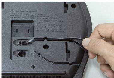
Plug in the Handset cable into the back of the base station. Put the cable into the cable groove.
