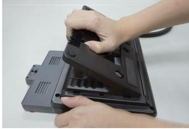
Mounting the stand at the media phone rear panel, make sure the latch on the stand and the hole on the media phone matched. Hold the stand and pull down gently.
